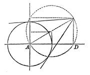
perpendicular to the axis of X and make it equal to y'. Join the extremity of the perpendicular and the origin A, and on this line as a diameter describe a circumference; the points P and P' in which it intersects the circumference of the given circle will be the
